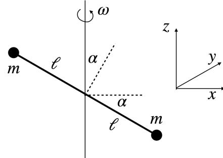
(a) Find all nine components of the inertia tensor for this coordinate system. (b) Find the (vector) angular momentum for the configuration as shown. (c) Find the kinetic energy for the configuration as shown. (d) Calculate the principal moments of inertia, and (e) find the principal axes for this configuration.
