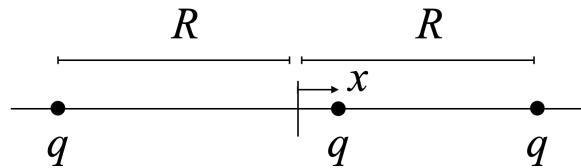
The outer two charges are fixed to the line, and are separated by a distance  $2R$ . The third charge can move along the line, where  $x$  measures its distance from the midpoint. Find the force on the middle charge in the limit  $x \ll R$  and use this to find the (angular) frequency “ $\omega$ ” for small oscillations about the midpoint if the middle charge has mass  $m$ .
