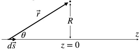
The vector  $d\vec{s} \times \vec{r}$  is perpendicular to the wire, that is, perpendicular to  $d\vec{s}$ , and also perpendicular to  $\vec{r}$ , which means it points azimuthally around the wire. Its magnitude is  $|d\vec{s}||\vec{r}|\sin\theta$  where  $\theta$  is the angle between  $d\vec{s}$  and  $\vec{r}$ . Therefore, if we let z measure the position along the wire with z = 0 being the point closest to the field point, then  $|d\vec{s}| = dz$  and
