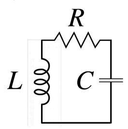
The initial charge on the capacitor is zero, and the initial current through the resistor is  $i_0$ . Find the current i(t) as a function of time, assuming that R is less than  $2\sqrt{L/C}$ .
