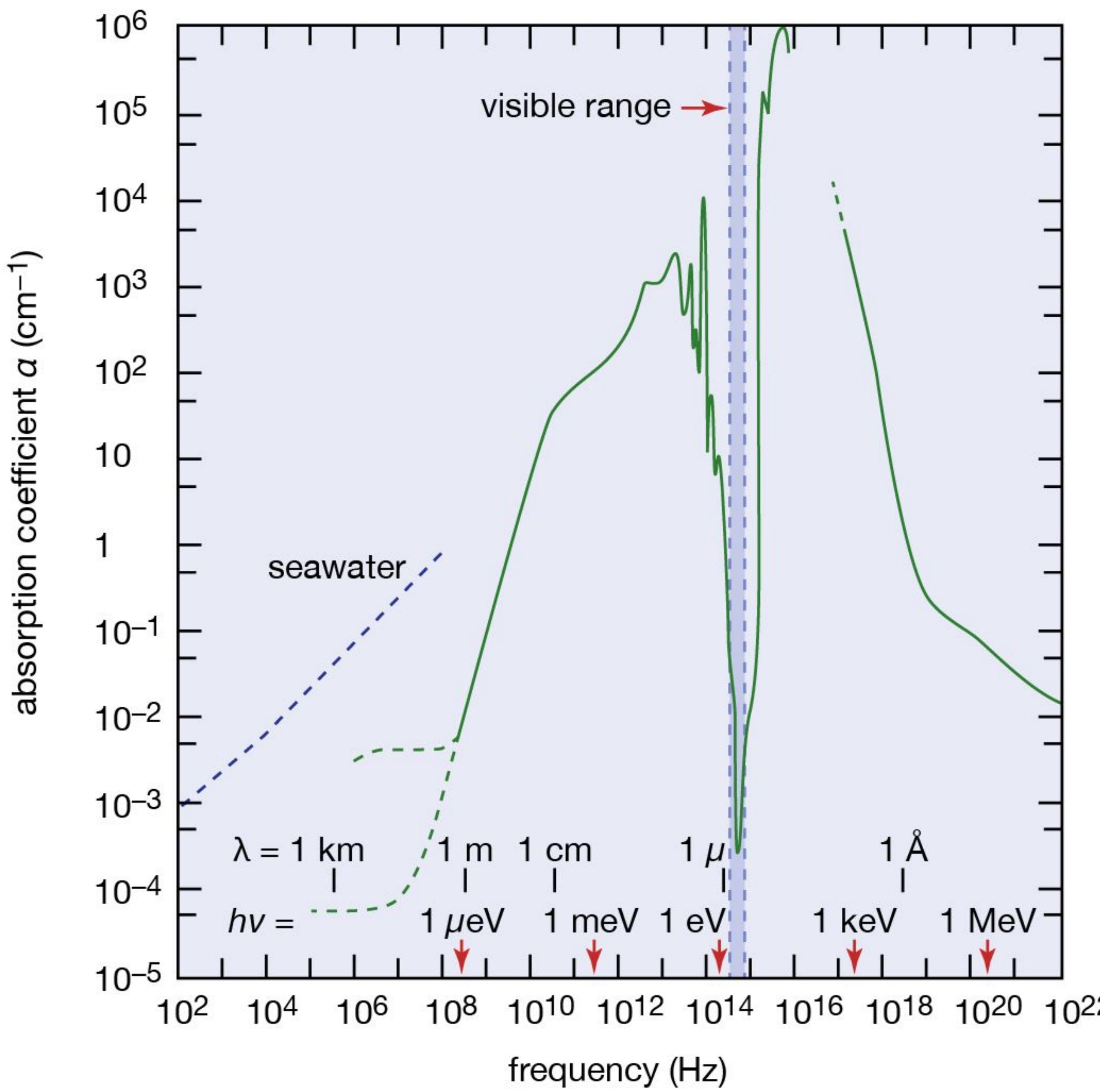
Also shown as abscissas are an energy scale (arrows) and a wavelength scale (vertical lines). The visible region of the frequency spectrum is indicated by the vertical dashed lines. The absorption coefficient for seawater is denoted by the dashed diagonal line at the left. The scales are logarithmic in both directions.
